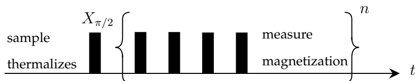
Figure 1.2: A typical NMR experiment, including initializing the state, a \pi/2 -pulse to measure magnetization in the xy -plane, and many repetitions of a pulse sequence and magnetization measurements. After each pulse sequence (between the brackets), the dynamics appear to have evolved due to an engineered Hamiltonian.
